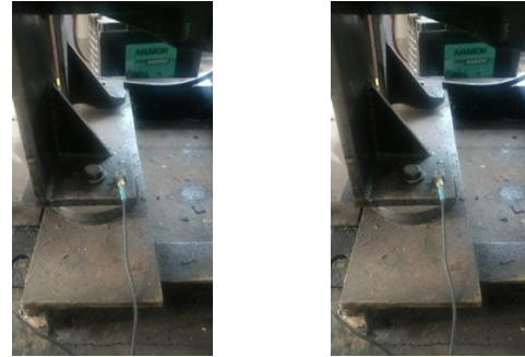
Figure 3. Tri-axial Sensor on left and right bottom of the engine with NR mount
