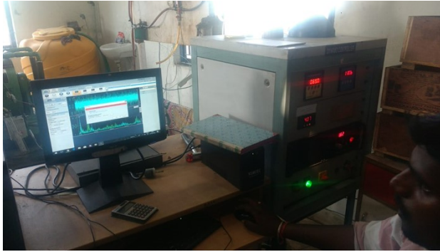
Figure 7. Dewesoft system shows the frequency spectrum analysis output
