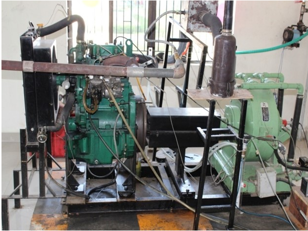
Figure 2. Two Cylinder 4 stroke DI Engine Experimental setup -
