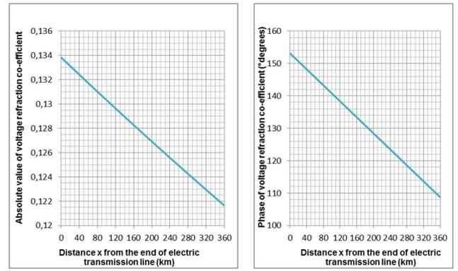
**Figure 3.** Absolute value (intensity) and phase (angle) of voltage refracted wave from the end towards the beginning of line i.e. along the direction the refracted wave moves (direction opposite to that of graph 1, i.e. left to right of electric power transmission line of figure 1)
