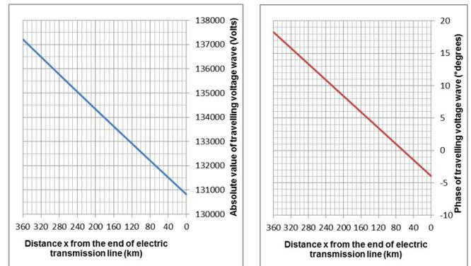
**Figure 2.** Absolute value (intensity) and phase (angle) of voltage travelling wave from the beginning towards the end of line i.e. along the direction the travelling wave moves (direction right to left of electric power transmission line of figure 1)
