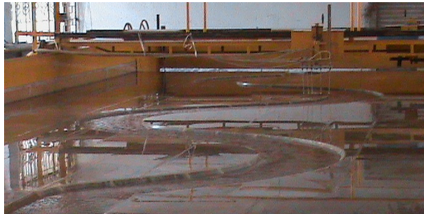
Photo 1: Details of meandering channel with the measuring equipments.
