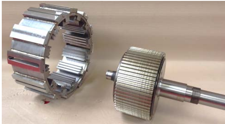
Figure 5. Reference Prototype (DSPM0) stator and rotor cores
