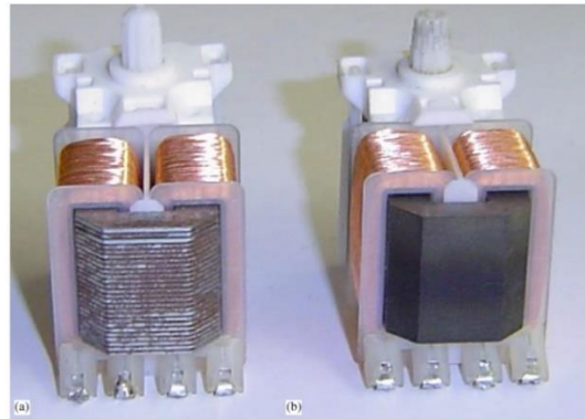
Figure 10. The stator of a synchronous electric motor made of (a) laminated silicon iron sheets, (b) soft magnetic compounds [63]
