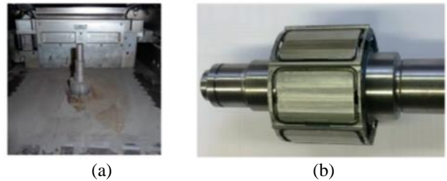
Figure 8. Additive manufacturing process (a) rotor active part and (b) shaft
