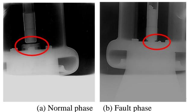
**Figure 8.** Transmission rod X-ray inspection images
