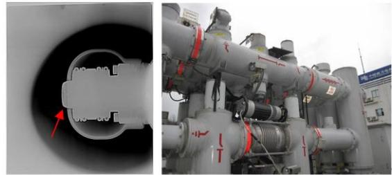
**Figure 6.** Schematic diagram of flaw position and photos (fault phase)
