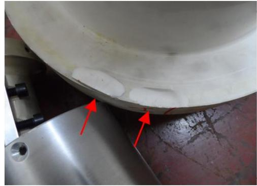
**Figure 12.** A photo of boss cracking and peeling off
