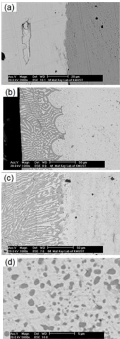
Figure 2. Morphologies and microstructures of Pb/Sn interphase diffusion solution layer for different holding times: (a)0h; (b)2h; (c)4h; (d)6h
