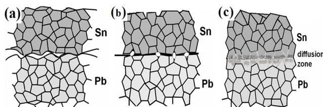
Figure 8. Formation of the interfacial transition zone for Pb/Sn diffusion welding
