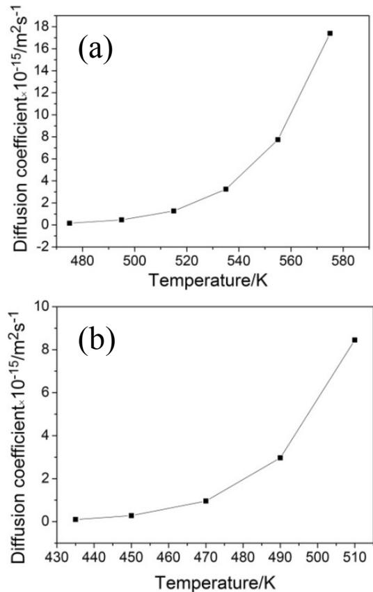
Figure 5. Relationship between self-diffusion coefficients of Pb (a) and Sn (b) and diffusion temperature
