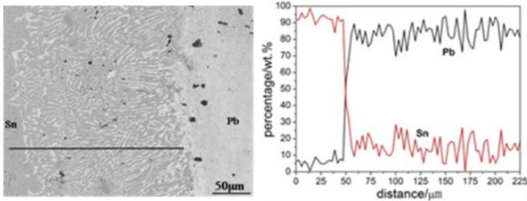
Figure 4. EDS microanalysis of the reaction zone at 503K for 2h
