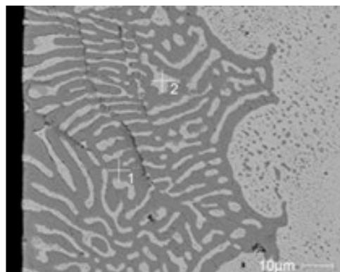
Figure 3. EDS microanalysis of the reaction zone at 503K and 2h
