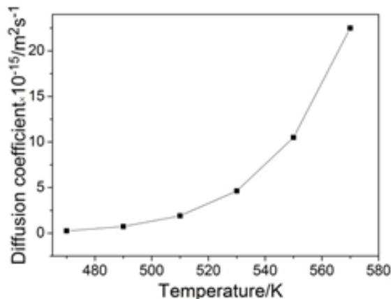
Figure 6. Relationship between diffusion coefficient of Sn in Pb substrate and diffusion temperature
