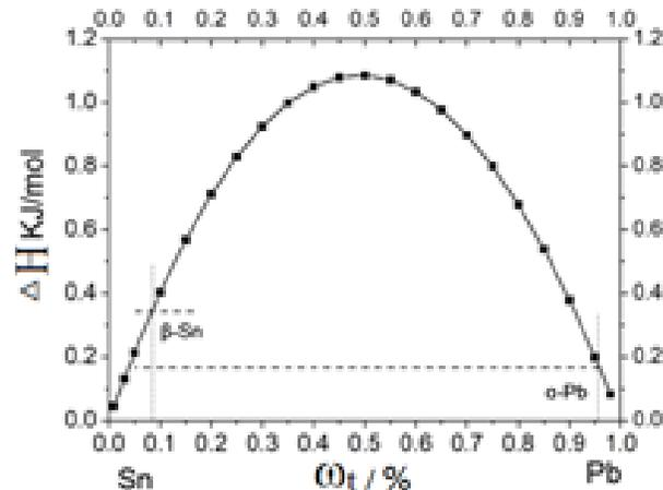
Figure 7. Relationship between  $\Delta H$  and the composition of the alloy
