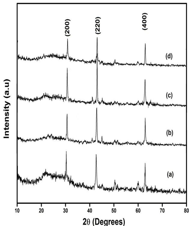
Figure 1. X-ray diffraction patterns of CdZnSe thin films electro-deposited at various bath temperatures: (a) 30°C (b) 50°C (c) 70°C and (d) 90°C.
