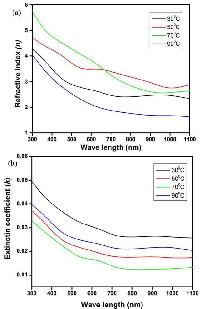
Figure 4. (a) Variation of refractive index ( $n$ ) and (b) extinction coefficient ( $k$ ) as a function of wavelength ( $\lambda$ ) for CdZnSe thin films obtained at various bath temperatures.
