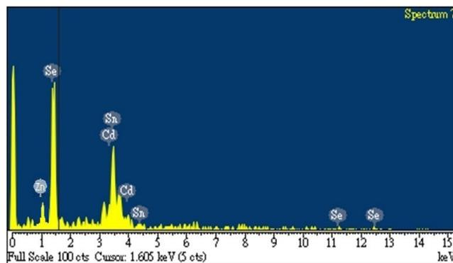
Figure 7. Typical EDX spectrum of CdZnSe thin film obtained at bath temperature 70°C.
