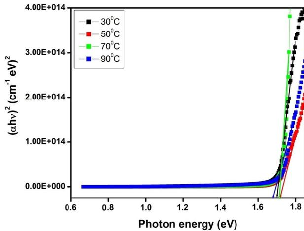
Figure 3. Plot of  $h\nu$  versus  $(\alpha h\nu)^2$  for CdZnSe thin films electrodeposited at various bath temperatures
