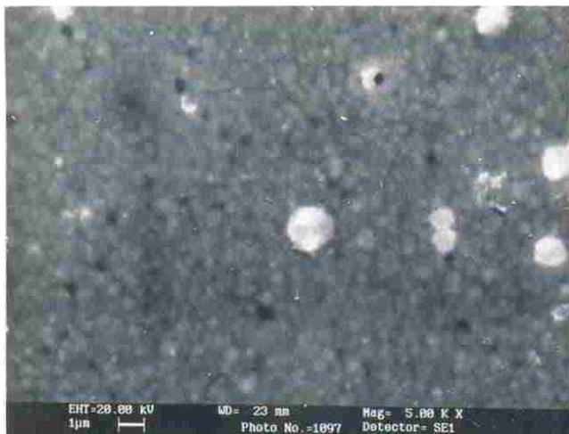
Figure 5. SEM picture of CdZnSe thin film obtained at bath temperature 70°C.
