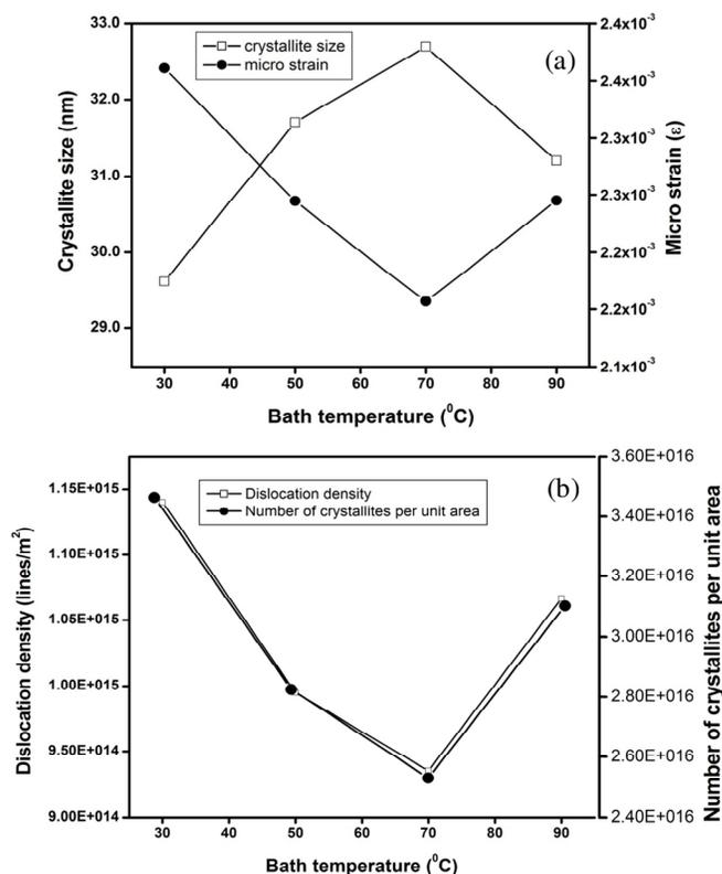
Figure 2. Microstructural properties of CdZnSe thin films for various bath temperatures (a) crystallite size and strain (b) dislocation density and number of crystallites per unit area
