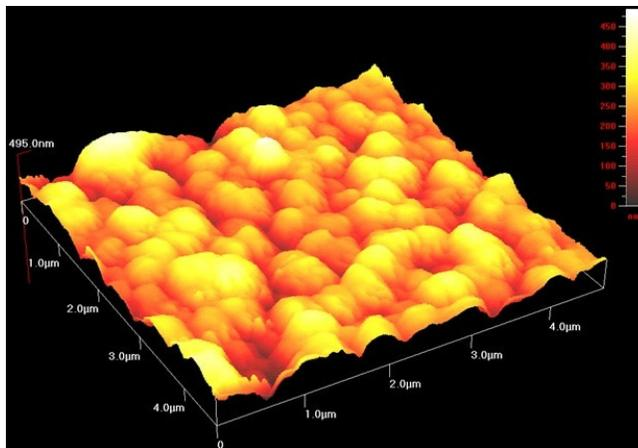
Figure 6. AFM image of CdZnSe thin film obtained at bath temperature 70°C.
