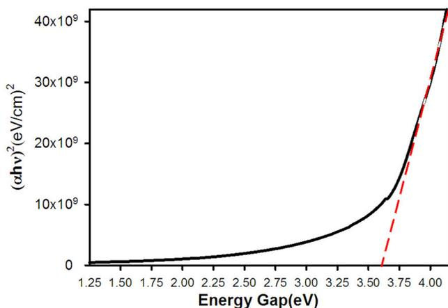
Figure 7. The ZnS energy band gap measurement
