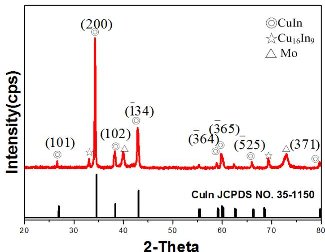
Figure 2. The XRD of the Cu-In film on top of Mo glass
