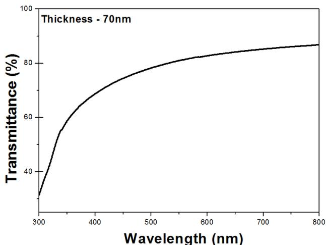
Figure 6. The transmittance of the ZnS film
