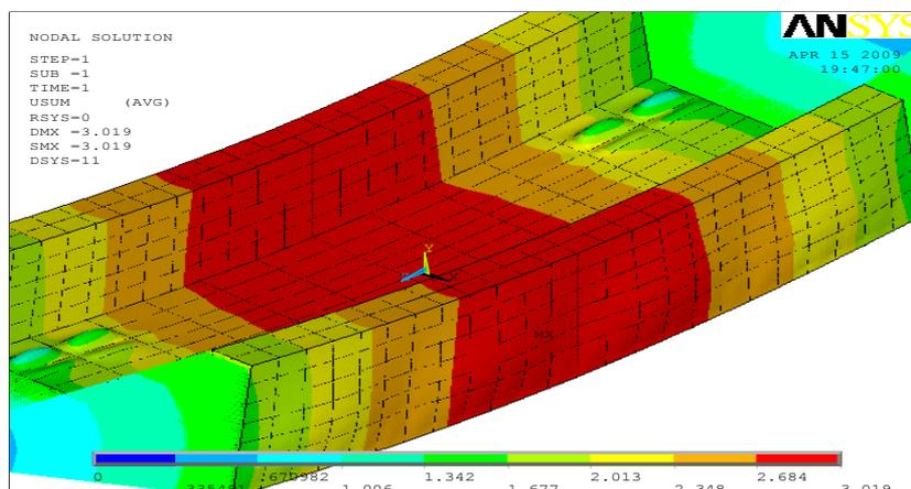
Figure 2. The deformation map in the fourth state
