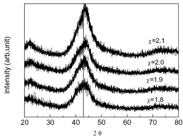
Figure 1: X-ray diffraction patterns of ball-milled  $\text{Mg}_{1.9}\text{Cu}_{0.1}\text{Ni}_\chi$  ( $\chi = 1.8, 1.9, 2.0, 2.1$ ) alloys.
