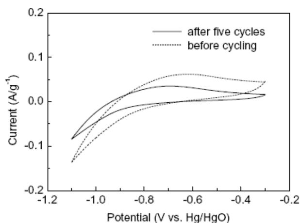
Figure 4: Cyclic Voltammograms of Mg<sub>1.9</sub>Cu<sub>0.1</sub>Ni<sub>1.9</sub> alloy electrode. Scan rate: 10 mV/s
