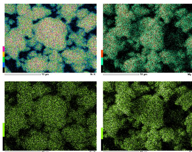
Figure 5: SEM image and concentration distributions of Mg, Ni, Cu and O in Mg<sub>1.9</sub>Cu<sub>0.1</sub>Ni<sub>1.9</sub> after five cycles.
