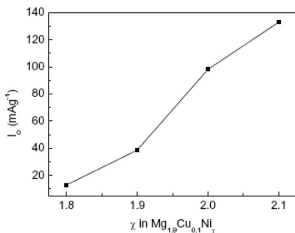
Figure 9: Variation of exchange current density with  $\chi$  in  $\text{Mg}_{1.9}\text{Cu}_{0.1}\text{Ni}_\chi$ .
