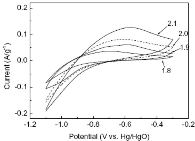
Figure 6: Cyclic Voltammograms for  $Mg_{1.9}Cu_{0.1}Ni_{\chi}$  ( $\chi = 1.8, 1.9, 2.0, 2.1$ ) alloy electrodes after 5 cycles. Scan rate: 10 mV/s
