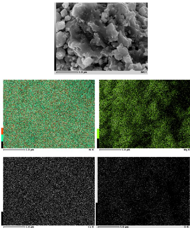
Figure 2: SEM image of as-received  $Mg_{1.9}Cu_{0.1}Ni_{1.9}$  alloy and Mg, Ni, Cu and O distribution in the alloy.
