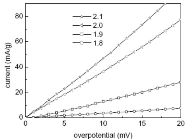
Figure 8: Linear polarization curves of  $Mg_{1.9}Cu_{0.1}Ni_{\chi}$  ( $\chi = 1.8, 1.9, 2.0, 2.1$ ) alloy electrodes after 15 cycles at 20 % depth of discharge.
