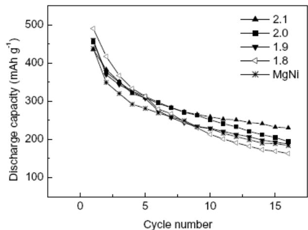
Figure 3: Discharge capacity via cycle number for  $Mg_{1.9}Cu_{0.1}Ni_{\chi}$  ( $\chi = 1.8, 1.9, 2.0, 2.1$ ) and MgNi alloy negative electrodes.
