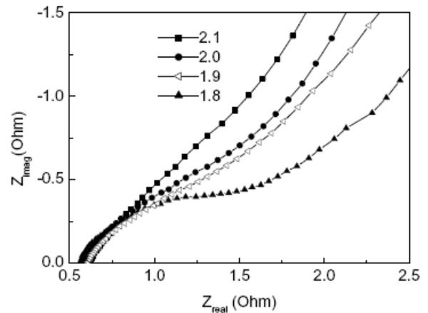
Figure 7: Electrochemical impedance spectra of  $Mg_{1.9}Cu_{0.1}Ni_{\chi}$  ( $\chi = 1.8, 1.9, 2.0, 2.1$ ) alloy electrodes after 15 cycles at 80 % depth of discharge.
