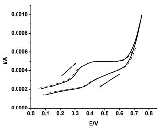
Figure 4. Matching between experimental (——) and simulated voltammograms (.....) of CT complex at a sweep rate of 0.5 V s<sup>-1</sup> and T = 25 °C
