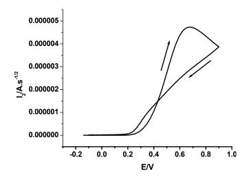
Figure 3. Kinetic convoluted current I<sub>2</sub> of CT complex at platinum electrode, sweep rate of 0.5 V s<sup>-1</sup>, T = 25 °C.
