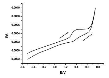
Figure 1. Cyclic voltammogram of charge transfer complex of 4,4'-bipyridine with benzoquinone derivative at platinum electrode, sweep rate 0.5 Vs<sup>-1</sup>, T = 25 °C
