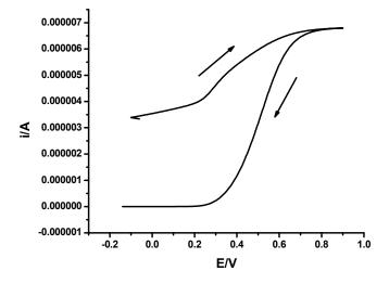
Figure 2. Convoluted current of investigated CT complex at platinum electrode, sweep rate  $0.5 \text{ V s}^{-1}$ , T = 25 °C.
