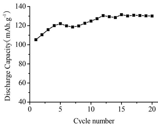
Figure 5. Cyclic performance of  $MgMnSiO_4$  tested at  $10 \text{ mA} \cdot \text{g}^{-1}$  at  $25 \text{ }^\circ\text{C}$
