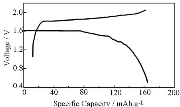
Figure 4. Typical charge/discharge curves of MgMnSiO<sub>4</sub> electrodes.
