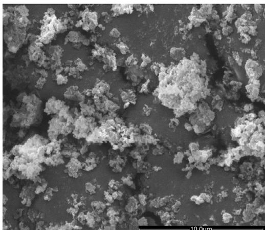
Figure 2. SEM image of MgMnSiO<sub>4</sub>
