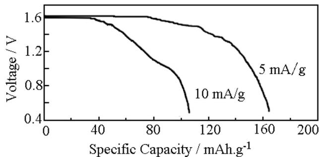
Figure 3. The voltage profiles of MgMnSiO<sub>4</sub> at 5 and 10 mA·g<sup>-1</sup> at 25 °C
