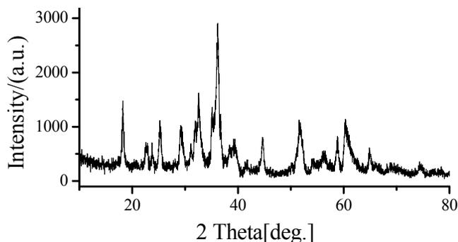
Figure 1. The XRD patterns of MgMnSiO<sub>4</sub> sample
