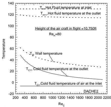
Fig3: Variation of Hot and cold fluid temperatures at a height 10,750 ft
