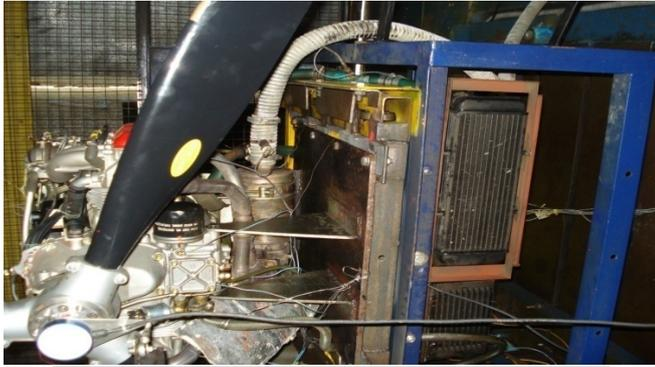
**View of the Engine Oil Heat Exchanger**
