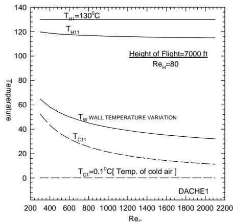
Fig2. Variation of hot and cold fluid temperatures at height of 7000 ft
