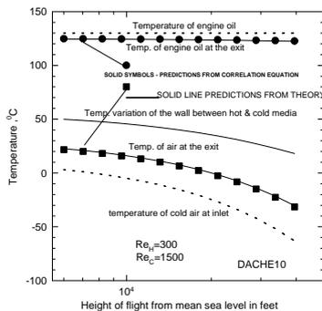
Fig 11 Variation of salient temperatures with height of flight
