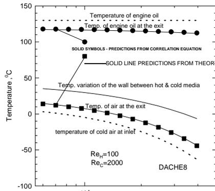
Fig 9 Variation of salient temperatures with height of flight
