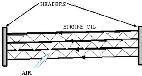
**Fig 1. SCHEMATIC OF CROSS FLOW UNMIXED ENGINE OIL HEAT EXCHANGER**
