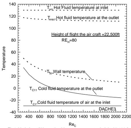
Fig4: Variation of Hot and cold temperatures at a height 22,500 ft
