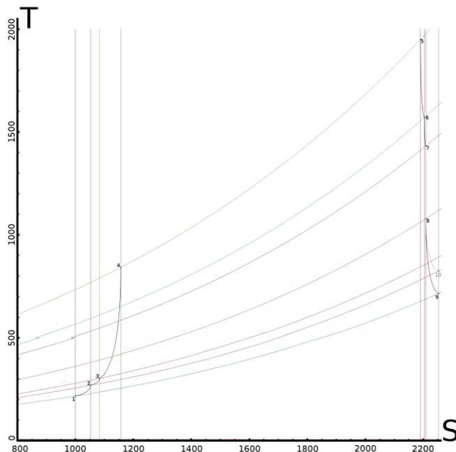
Figure 3 Temperature T [K], Entropy S diagram of a very high performance military turbofan engine
