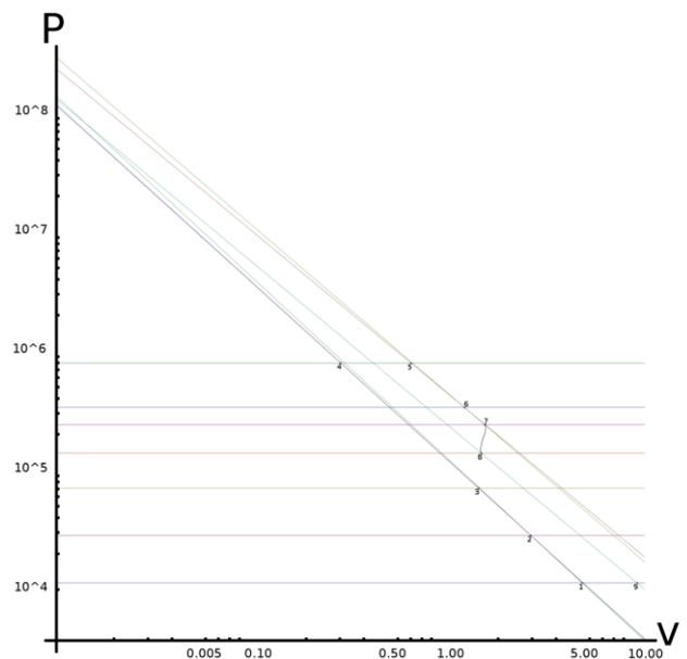
Figure 2 – pressure (p) [Pa], specific volume (V)[m³/kg] log-log diagram of a very high performance military turbofan engine
