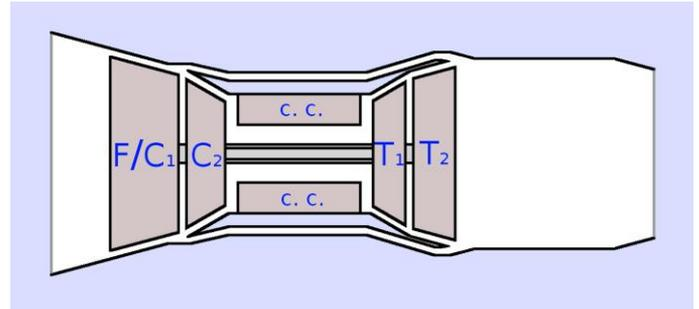
Figure 1 - Scheme of a typical turbofan engine
