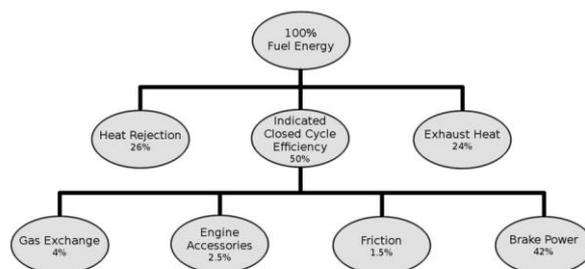
Figure 4: Energy audit for a typical diesel engine
