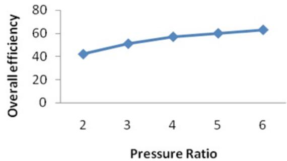
Figure 5: turbodiesel efficiency with compressor pressure ratio
