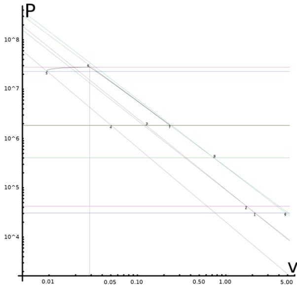
Figure 8: pressure (p) [Pa], specific volume (V)[m³/kg] log-log diagram of the turbocompound engine
