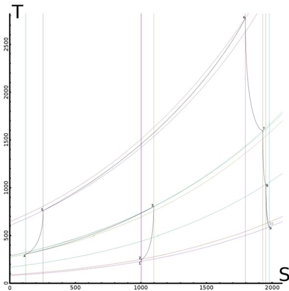
Figure 9 Temperature/Entropy diagram of the turbocompound engine
