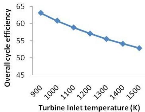
Figure 6: turbodiesel efficiency with exhaust temperature
