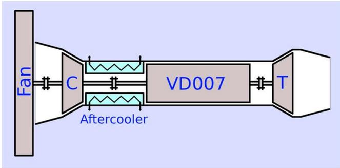
Figure 7 - Scheme of the Diesel-Brayton turbocompound engine
