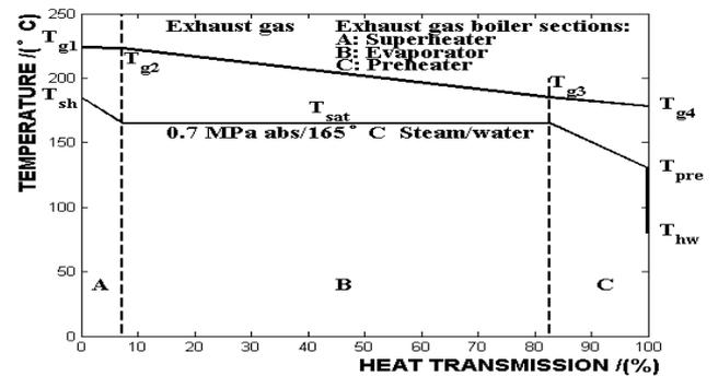
Figure 4 Temperature/heat transmission diagram of exhaust gas boiler
