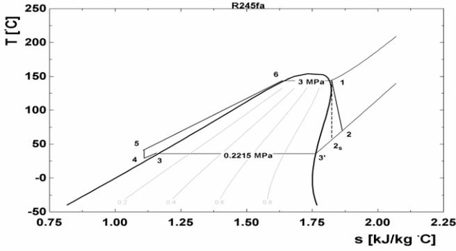
Figure 7 R245fa T-S diagram
