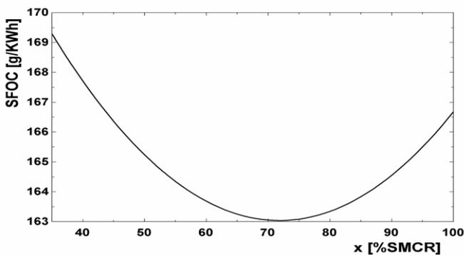
Figure 2 Specific Fuel Oil Consumption(SFOC) of intelligent marine diesel engine—10S90ME of MAN B&W
