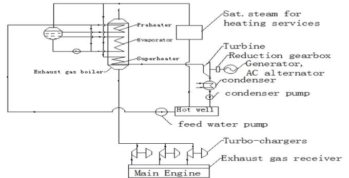
Figure 3 Ordinary Rankine Cycle(RC) conceptual waste heat recovery system diagram
