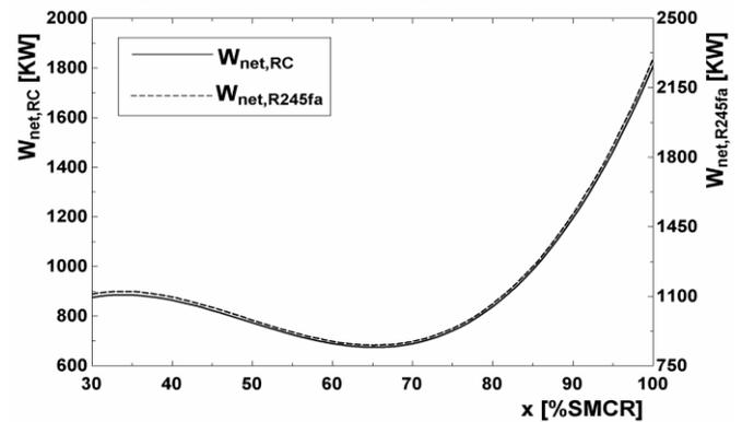
Figure 12 Net power output variation with main engine load
