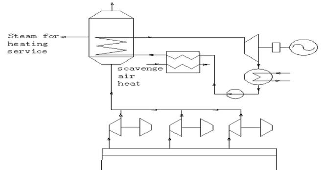
Figure 6 Organic Rankine Cycle (ORC) conceptual waste heat recovery system diagram
