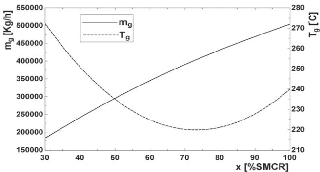
Figure 1 Exhaust gas temperature and amount after turbocharger of intelligent marine diesel engine—10S90ME of MAN B&W
