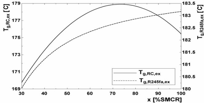
Figure 8 Exhaust gas exit temperature variation with main engine load
