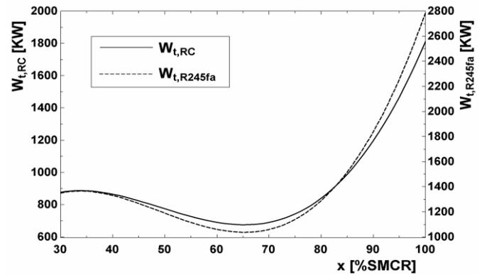
Figure 11 Turbine power output variation with main engine load
