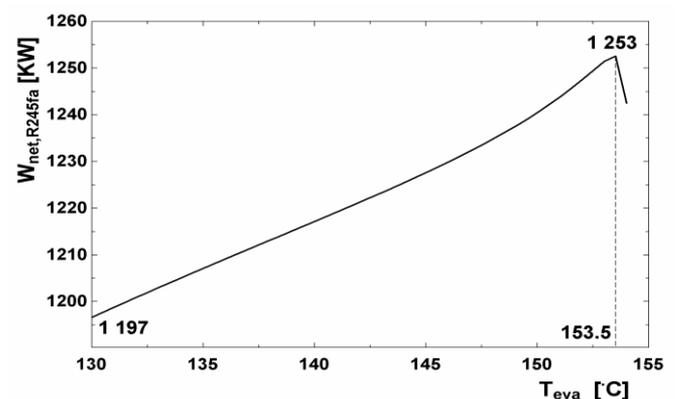
Figure 13 Net power output variation with evaporation temperature
