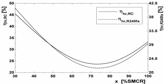
Figure 9 Heat recovery efficiency variation with main engine load
