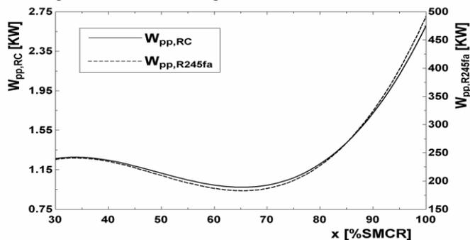
Figure 10 Exhausted electricity by pump variation with main engine load
