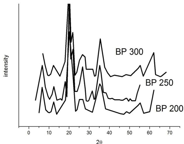
Figure 1. Diffractogram of Pillared Bentonite
