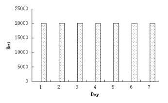
Figure 7. Effect of the testing time on the resistance value due to MOP reaction using immuno-sensors
