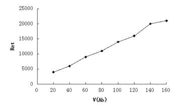
Figure 5. Effect of the concentration of the binding antibodies (20  $\mu$ L per time) on the resistance of the electron change transfer
