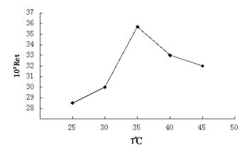
Figure 4. Effect of the temperature of antibody modification on the resistance of electron transfer due to the detection of the antigen
