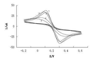
Figure 1. Cyclic voltammogram (curves of (1) bare gold electrode, (2) 3-mercaptopropionic acid modified, (3) EDC-NHS activation, (4) Antibody firstly modified by 20iL of KTHC and (5) Sufficient modified antibodies)
