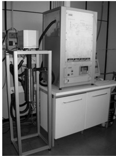
Figure 2. Photograph of the measuring chamber and balance (left) and gas dosing system (right)
