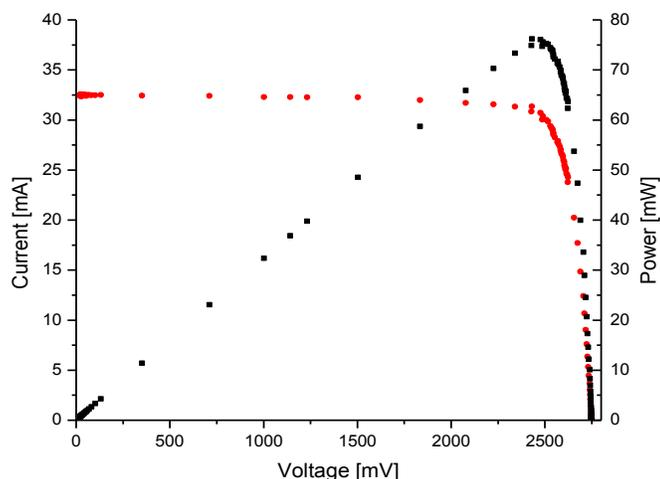
Figure 8. I-V curve of a photovoltaic cell with concentrator lens
