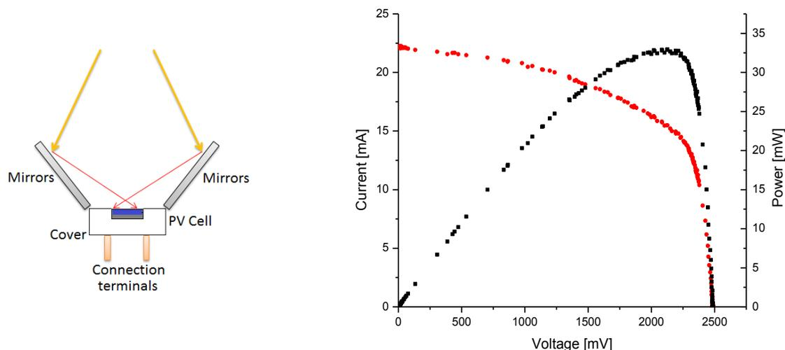
Figure 7. The I-V curve of a PV concentrator cell with mirrors
