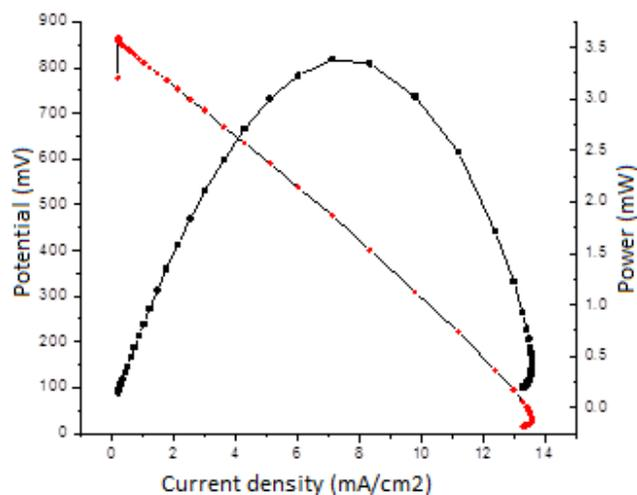
Figure 9. The E-I curve of the PEM fuel cell
