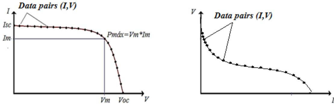
Figure 1. Typical I-V curves for energy converters a) photovoltaic cell, b) fuel cell
