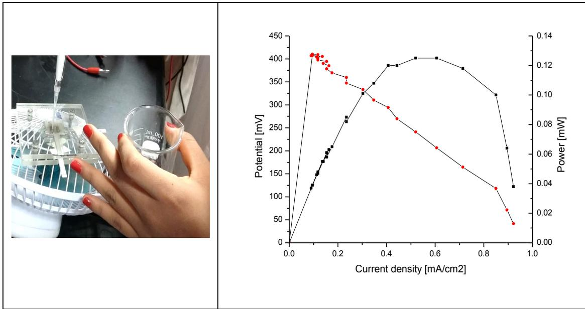
Figure 10. The E-I curve of the experimental direct ethanol fuel cell
