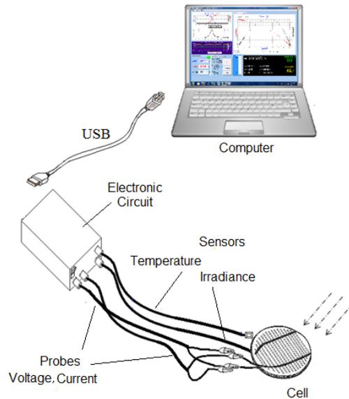
Figure 5. The prototype of the electronic system for acquiring data from the energy conversion devices
