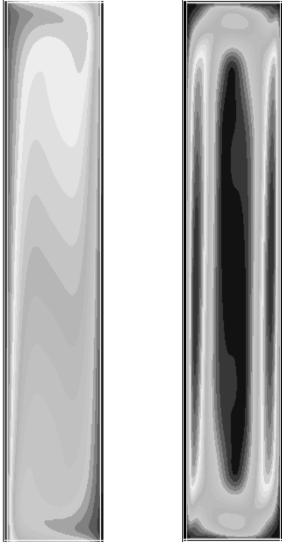
Fig. 4 – Temperature (left) and velocity (right) for 5 cm thick cavity, \Delta T=10 K, T_m=288 K.
