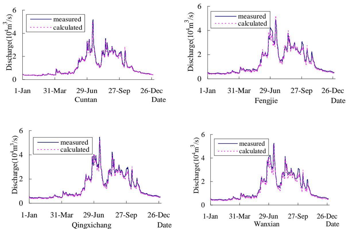
**Figure 3.** The comparison between measured discharge and calculated discharge of some stations in 2000
