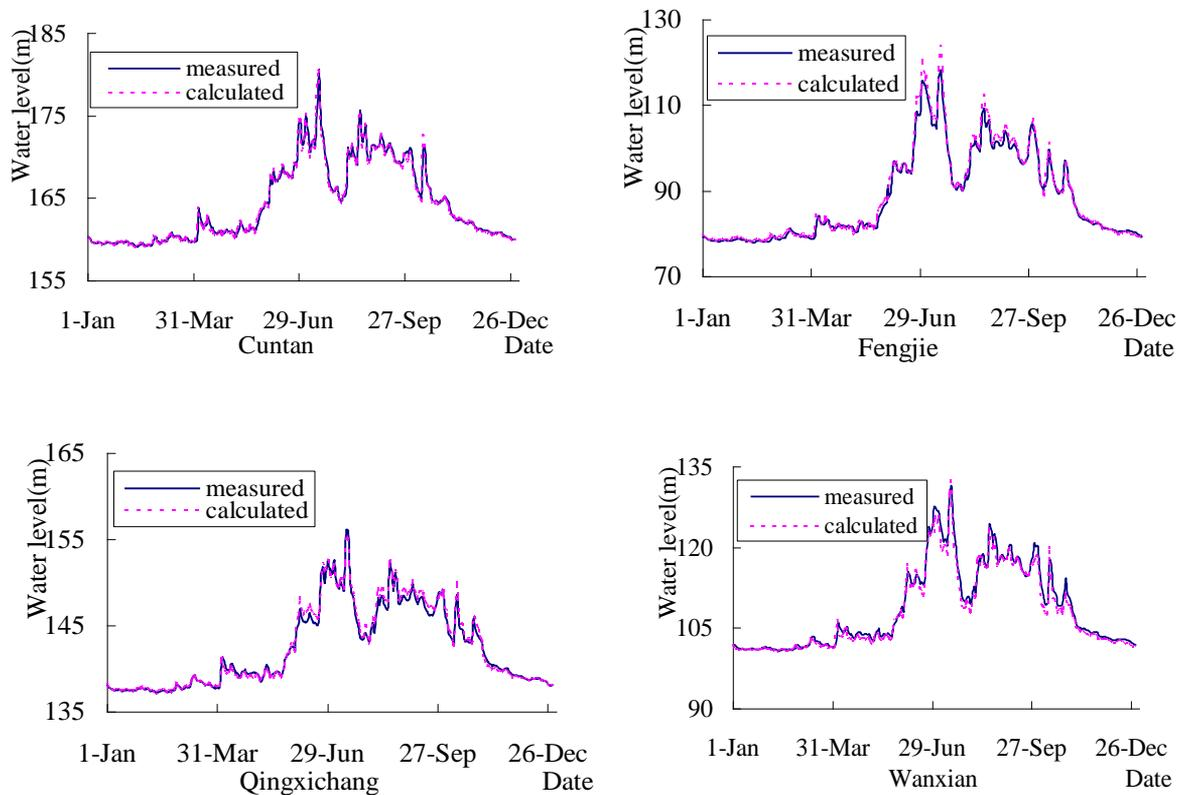
**Figure 2.** The comparison between measured water-level and calculated water-level of some stations in 2000
