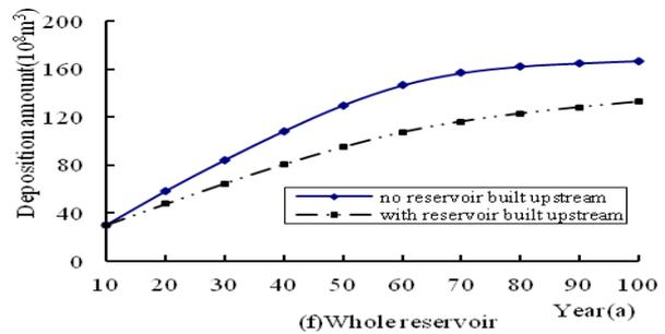
Figure 5. The deposition developing in TGR with reservoirs built upstream or not
