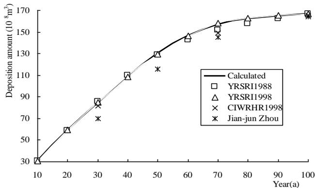
**Figure 4.** The deposition developing in TGR
