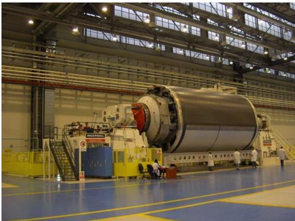
**Figure 17:** Tape winding (Courtesy of Boeing).
