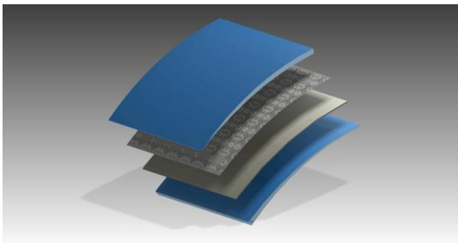
**Figure 11:** Exploded view of the core, network monitoring and polyurethane insulation.
