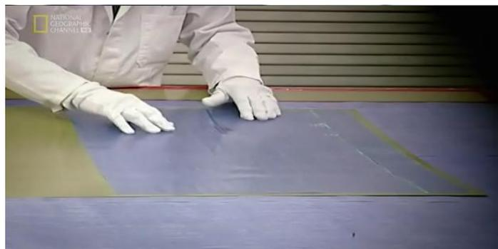
**Figure 15:** GLARE layers (1) (Courtesy of Airbus Industries).
