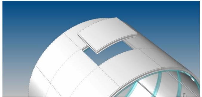
**Figure 19:** C-triplex panel assembly in an airplane fuselage plug.
