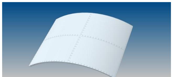
**Figure 20:** Four bordering C-triplex panels forming a cylindrical-shape part of the fuselage.
