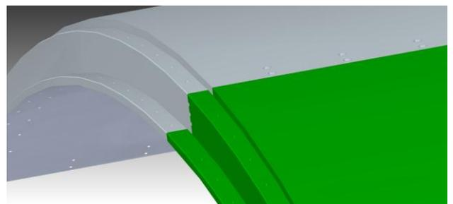
**Figure 21:** Male-female C-triplex panels coupling.
