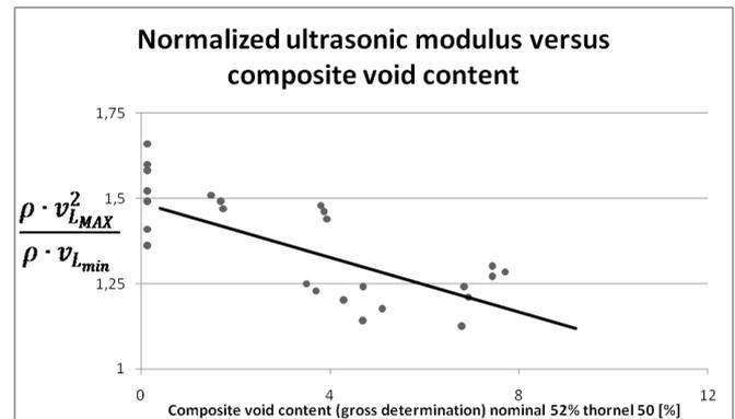
Figure 3: Normalized elastic modulus vs. void content. A void content up to 2% is normal [1].
