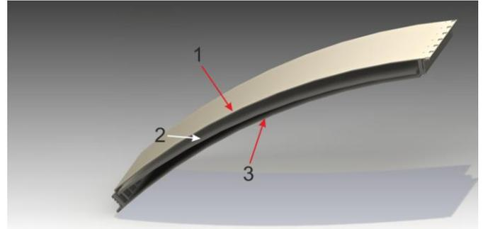
Figure 6: Cutaway drawing of the C-triplex panel. Protective shells (1 and 3) enclose the core structure (2).
