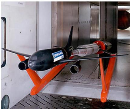
Figure 2. A310 model on the S2MA twin sting supports
