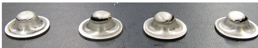
Figure 7: Specimens after deep-drawing test (340°C) Experimental velocity (a) 0.1 mm/s, (b) 0.5 mm/s, (c) 1.0 mm/s, (d) 1.5 mm/s.
