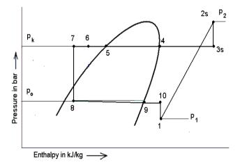
Figure 1. Actual vapor compression cycle for theoretical thermodynamic analysis
