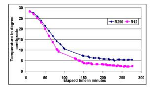
Figure 7. Temperature profiles of refrigerants in upper compartment during ice making test
