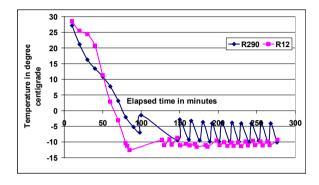
Figure 6. Temperature profiles of refrigerants in Freezer during ice making test
