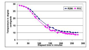
Figure 8. Temperature profiles of refrigerants in lower compartment during ice making test
