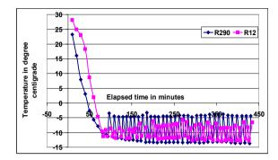
Figure 3. Temperature profiles of refrigerants in Freezer during no load performance test
