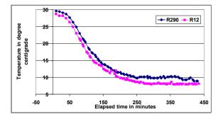
Figure 5. Temperature profiles of refrigerants in lower compartment during no load performance test
