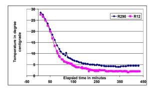
Figure 4. Temperature profiles of refrigerants in upper compartment during no load performance test
