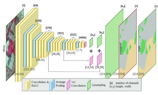
Figure 1. VGG-19 architecture model
