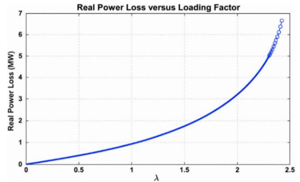
Figure 8. Dependence of real power loss on the loading factor \lambda
