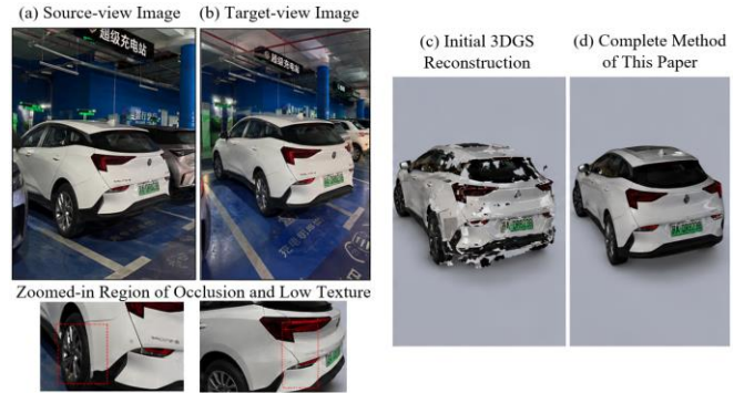
Figure 5. Implementation effect of multi-view image registration and 3D visual reconstruction in low-texture and view occlusion scenes
