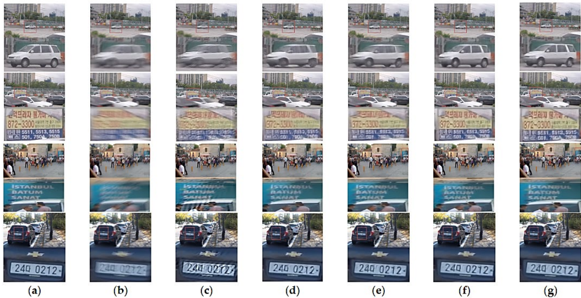
Figure 8. Test results in GoPro Set: (a) ground truth (sharp images), (b) input blurred images, (c) Restormer (transformer-based method), (d) Attention-Adaptive + Deformable Conv Module, (e) DeblurGAN-v2 (GAN-based Deblurring), (f) Scale-Recurrent Network (SRN), and (g) proposed deblurring method
