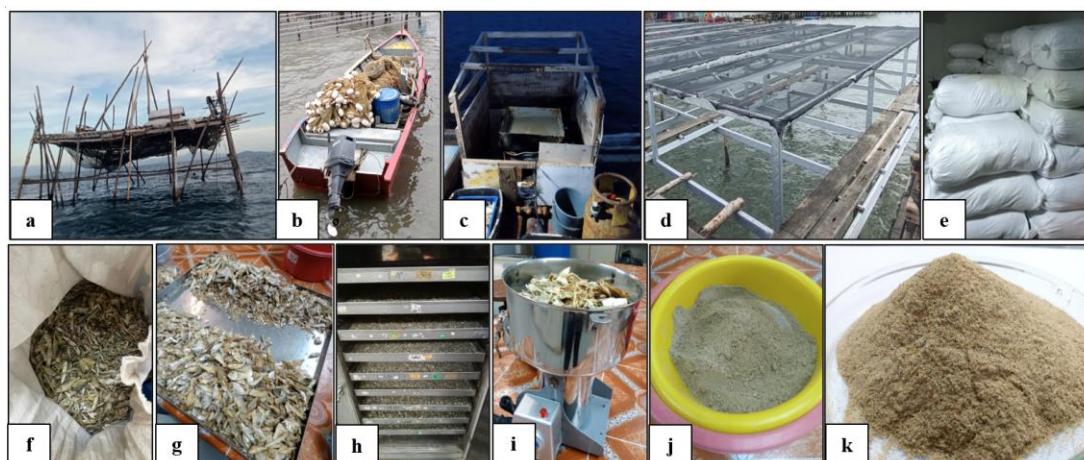
Figure 2. Processing pathway from anchovy harvesting to fishery by-catch meal (FBCM) production
