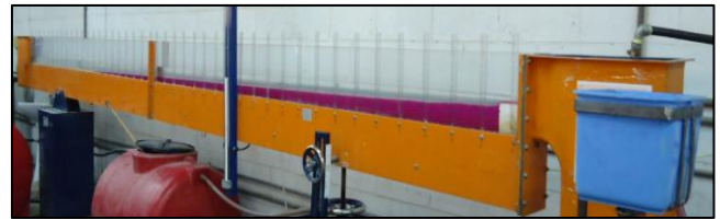
Figure 1. Salt wedge propagation case study in laboratory
