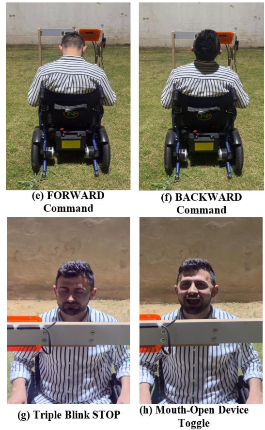
Figure 5. Practical operational conditions of the proposed facial-gesture control system: (a) prototype front/neutral view, (b) prototype rear/neutral view, (c) LEFT command, (d) RIGHT command, (e) FORWARD command, (f) BACKWARD command, (g) triple-blink STOP command, and (h) sustained mouth-opening gesture used to toggle the auxiliary device between ON and OFF states
