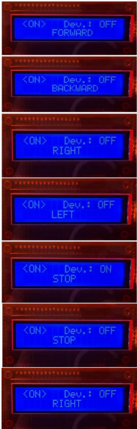
Figure 6. Real-time LCD1602 feedback display for wheelchair navigation and auxiliary device control states Table A1 summarizes a comparison of the proposed system with representative assistive wheelchair control approaches in
