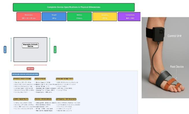
Figure 12. Physical device specifications and dimensions. Left: Dimensional profile (280 mm × 95 mm × 65 mm) with color-coded annotations (red = length, blue = depth, green = profile)
