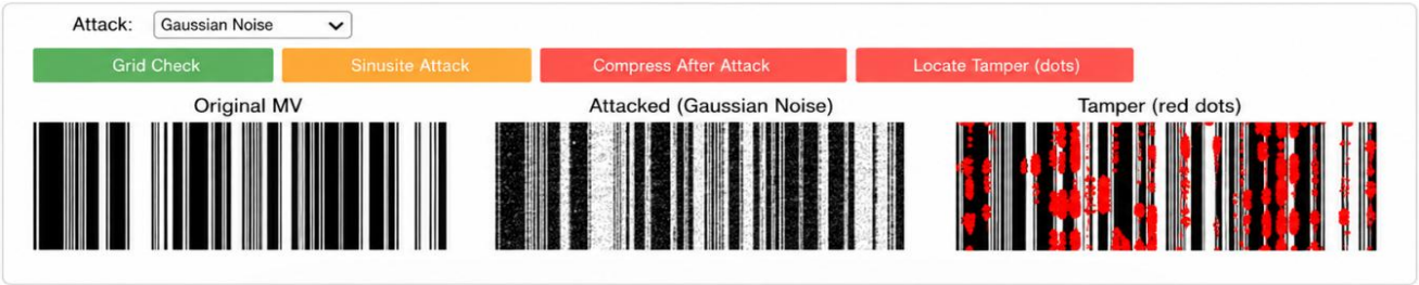
Figure 5. Tamper-localization output showing red markers over the affected regions
