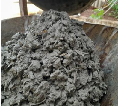
Figure 4. Drink cans fibers in concrete
