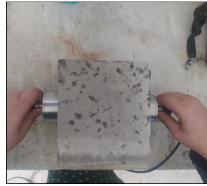
Figure 6. Ultrasonic velocity test
