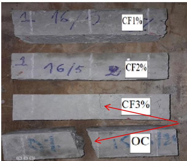
Figure 17. Flexural tensile failure behaviour of the 04 test specimens
