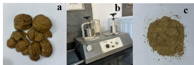
Figure 1. Walnut shell used in the experiment (a) before grinding, (b) planetary ball mill machine, and (c) after grinding
