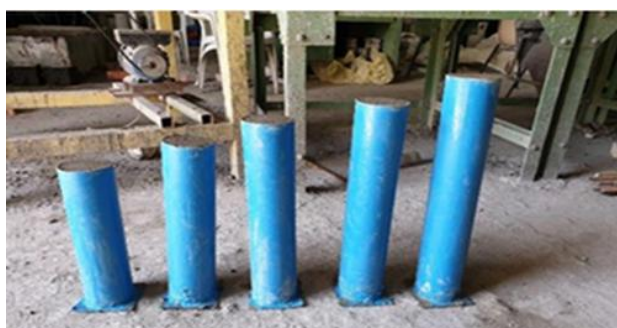
Figure 2. Columns after being filled with geopolymer concrete
