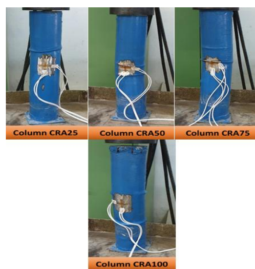
(b) Failure modes of steel tubular columns with different percentages of recycled concrete aggregate (RCA)
