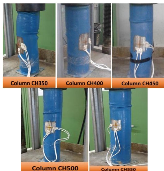
(a) Failure modes of steel tubular columns with different heights (continuous)
