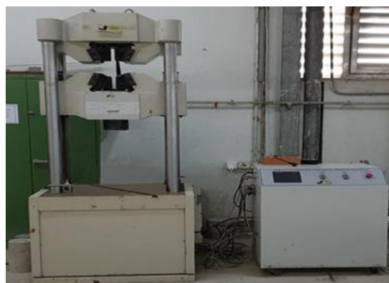
Figure 3. Testing machine for steel tubular columns
