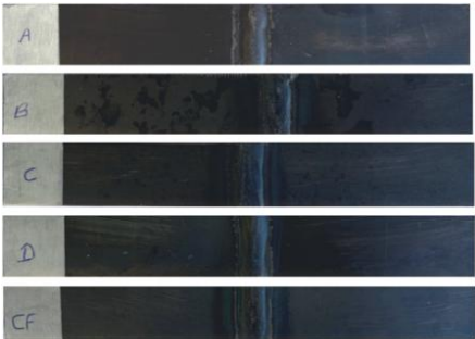
Figure 4. Samples welded using submerged arc welding (SAW) with different flux grades
