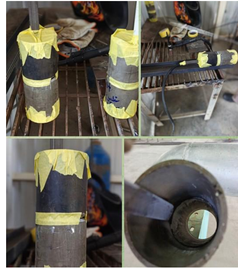
Figure 5. The gas shielding and filler application procedure
