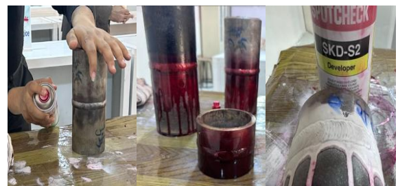
Figure 6. The procedure of liquid penetrant testing (PT)
