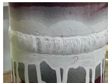
Figure 9. Visual inspection and liquid penetrant testing (PT) results
