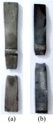
Figure 12. Representative tensile-tested specimens after fracture: (a) Stainless steel–stainless steel (SS–SS) joint and (b) carbon steel–stainless steel (CS–SS) joint
