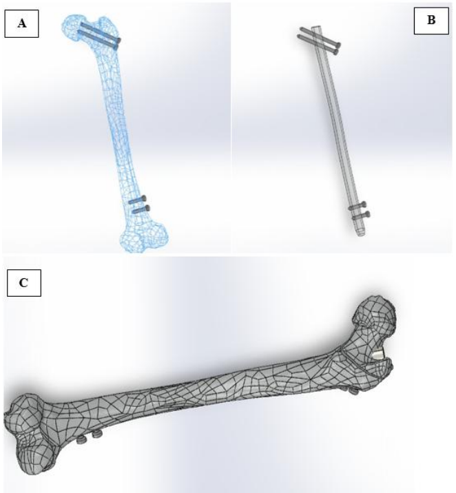
Figure 1. SOLIDWORKS femur bone design (A) the four screws locations, (B) the main implant bar with its fixture screws, and (C) the complete bone with all parts
