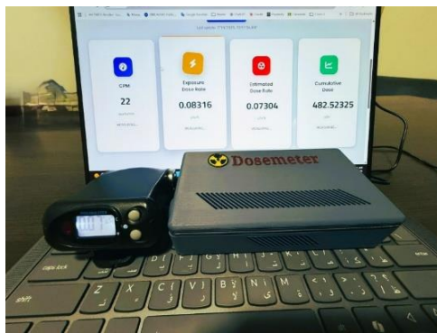
Figure 5. Validations of the proposed dosimeter with the reference electronic dosimeter Polimaster
