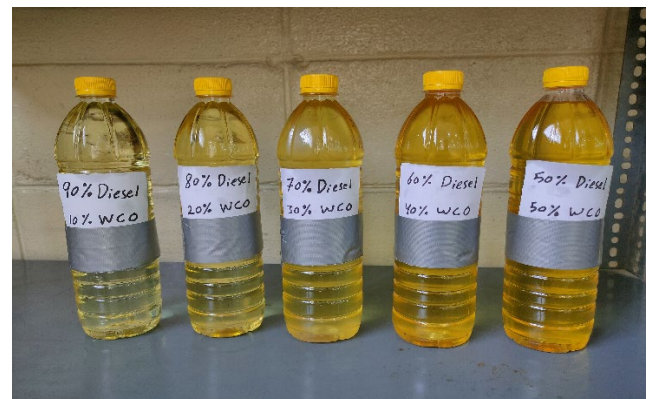
Figure 2. Prepared waste cooking oil (WCO) biodiesel–diesel blends (B10–B50) used in the experimental investigation
