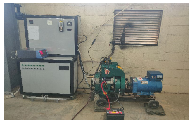
Figure 3. Photograph of the experimental diesel engine test rig
