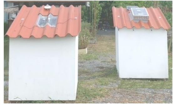
Figure 3. The Skylight Thermoelectric Roof Solar Collector (STRSC) and simple fiber roof (SFR) model houses
