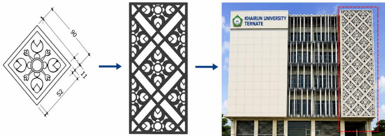
Figure 4. Type A academic sunscreen: Nutmeg-clove motif as a medium-porosity light-filtering facade element in the Integrated Lecture Building
