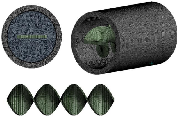
Figure 4. Mesh generation for the domain
