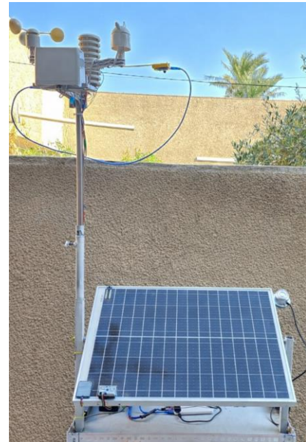
Figure 2. Real setup of the experimental system, including photovoltaic (PV) panel, weather station, and camera
