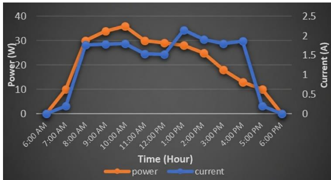
Figure 9. Daily variation of photovoltaic (PV) output power (W) and output current (A) from 6:00 a.m. to 6:00 p.m.
