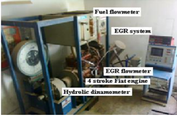
Figure 1. Photo of the experimental setup used in the tests
