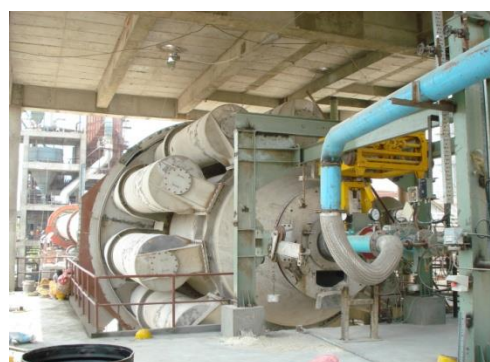
Figure 1. Satellite cooler with oil burner of rotary lime kiln
