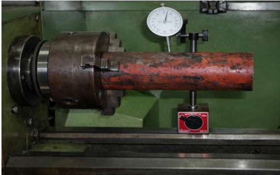
Figure 3. SCH40 pipe configurations prior to machining
