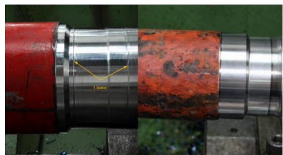
Figure 7. Surface roughness and chatter on the SCH40 pipe surface
