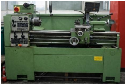
Figure 1. Emco Maximat V13 lathe used in the turning experiments
